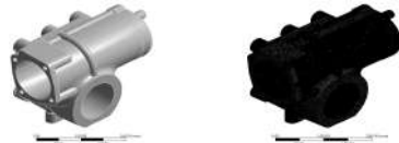
Fig. 2 Shape simplification and meshing of housing model
