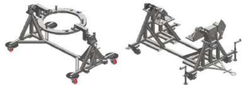
Fig. 1 Module stands of aircraft engine
