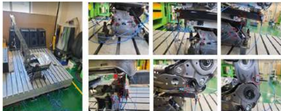
Fig. 1 Seat frame modal test settings
