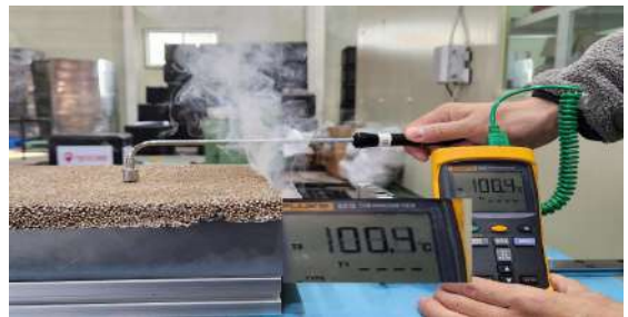
Fig. 1 Thermal insulation performance measurement test scene
