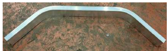
Fig. 3 Bending Products of Aluminum Extrusion Member
