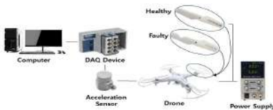
Fig. 1 Fault prediction big data collection system conceptual diagram
