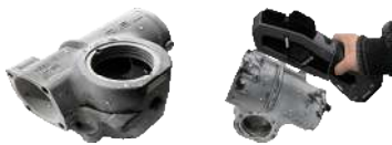
(a) Apply developer (b) 3D scanning
