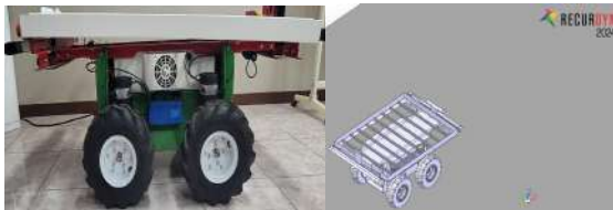
Fig. 1 Self-driving platform for transportation of agricultural materials
