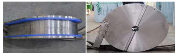
Fig. 2 Bending Mold of Aluminum Extrusion Member
