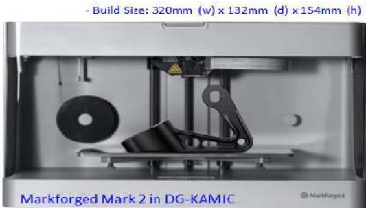
Fig. 1 Markforged Mark Two, 3D Printing with Continuous Fiber Reinforcement
