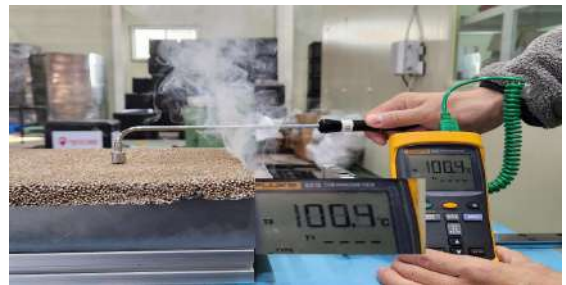
Fig. 1 Thermal insulation performance measurement test scene
