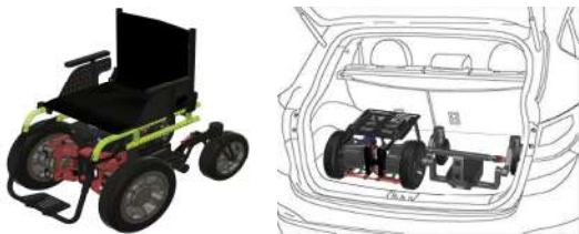
Fig. 1 Developed modular wheelchair (Todo Works社)
