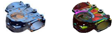
(a) complete origin setting for design and zoning to extract reference geometry
