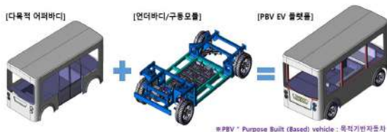
Fig. 1 Platform of Small Purpose Built Vehicle
