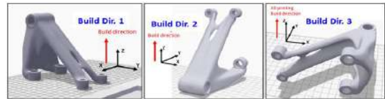
Fig. 3 Various build direction of a mechanical part
