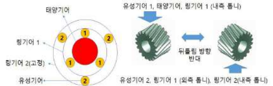
Fig. 1 Proposal of Planetary gear shape with double ring gear
