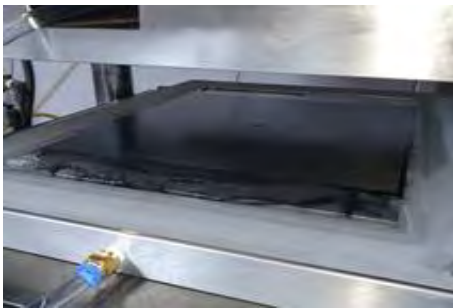
Fig. 1 Carbon Composite Specimens Containing GNP
