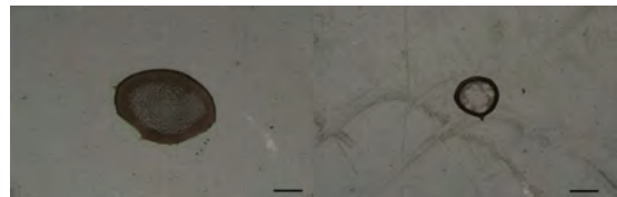
Fig. 2 Aggregate of organogel in 9:1 and 4:6 (UV curable material : lubricant) ratio. scale bar: 300μm
