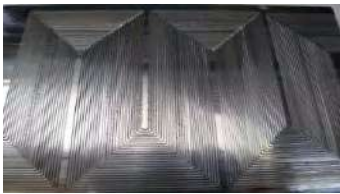
Fig. 1 Bipolar plates flow-path pitch machining
