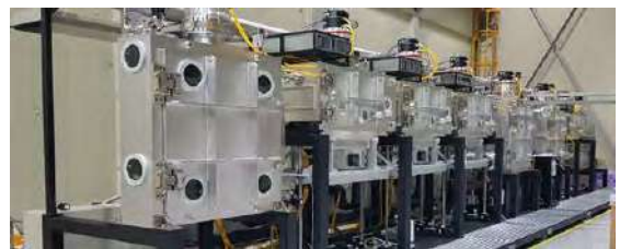
Fig. 2 Fabricated In-Line system for Buffer Layer Deposition
