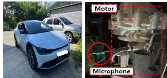
Fig. 1 The Test Car(left), Position of microphone(right)
