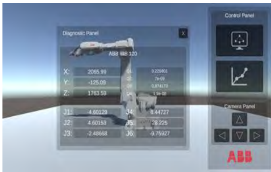
Fig. 1 Robot monitoring system GUI and panel displaying data for each axis and coordinates of the robot end-effector.
