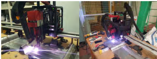
Fig. 1 Automatic welding machine for flat area(left) & corner area(right)
