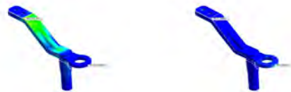
Fig. 2 The results of finite element analysis of gripper arm
