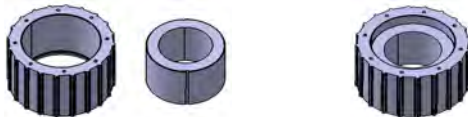
(a) Housing and stator (b) Assembled housing and stator Fig. 1 3D assembly shape of traction motor housing and stator
