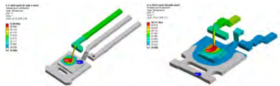
Fig. 2 TO-220,TO-252 Temperature Distribution
