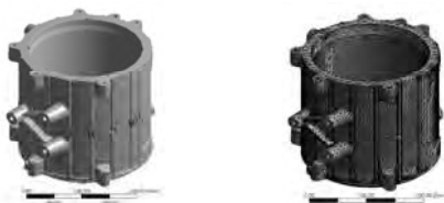
(a) Housing analysis model (b) Mesh model Fig. 1 Analysis model and mesh model of traction motor housing
