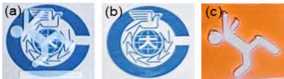
Fig. 1 Fabricated sliding motion shape surface (a) non-slippery surface (b) slippery surface (c) formation of liquid pattern by slippery property
