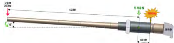
Fig. 3 Check the load on the connection link
