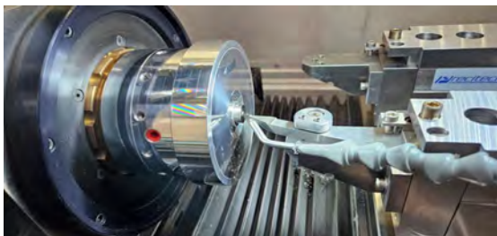
Fig. 1 Ultra precision machining of SUS329J1
