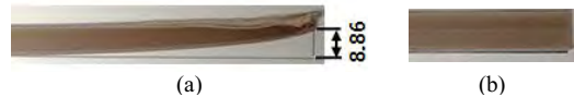
(a) Without AWC (b) AWC Dia. 50 Fig. 2 PEEK 3D printing thermal warpage(unit : mm)
