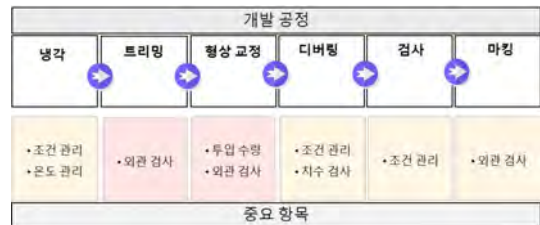
Fig. 1 Process flow diagram of die casting post-process
