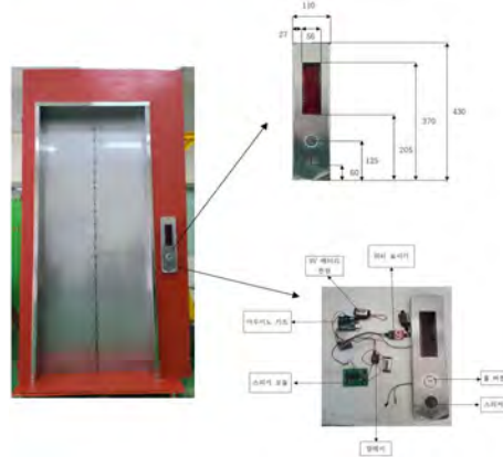
Fig. 2 Picture of EOD system using Arduino
