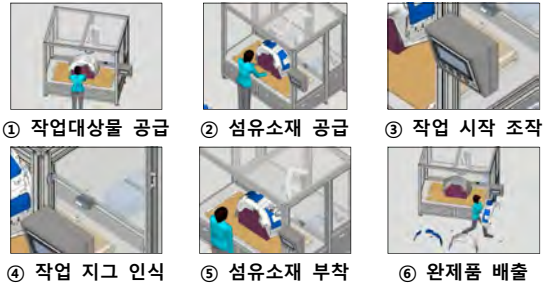
Fig. 2 Simulation of Process Flows Using Delfoi Robotics
