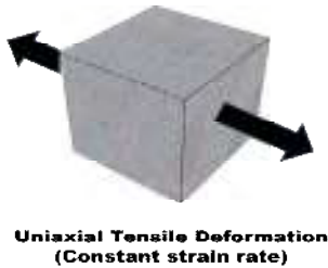
Fig. 1 Schematic diagram of uniaxial tensile simulation. Arrows represent the direction of elongation.
