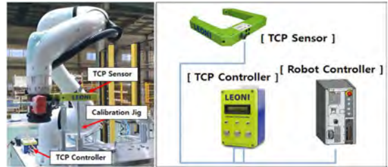
Fig. 2 Robot position calibration module with TCP sensor
