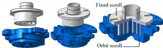
Fig. 1 Structure and assembly of scroll compressor
