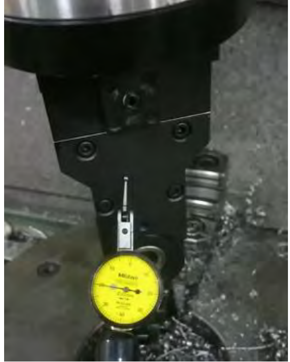
Fig. 3 Angle spindle idling test in vertical machining center
