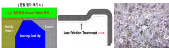
Fig. 1 Description of Low Friction Treatment Technology
