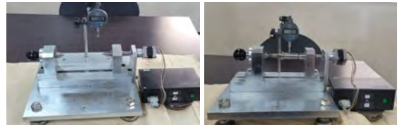
Fig. 3 Workpiece roundness measuring device(left) and device test(right)
