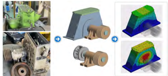
Fig. 3 Shot Blast Modeling and Finite Element Analysis
