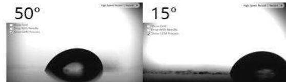
Fig 1. Left) water movements at original solar panel Right) water movements at Slippery surface solar panel
