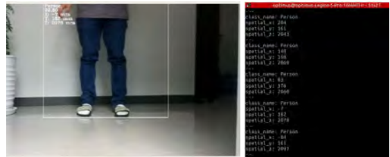
Fig. 1 Object(person) tracking(left). Real time publication of three dimensional position of object(person).
