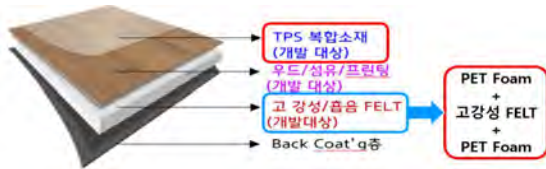
Fig. 1 Constituent layers of the Flat Floor
