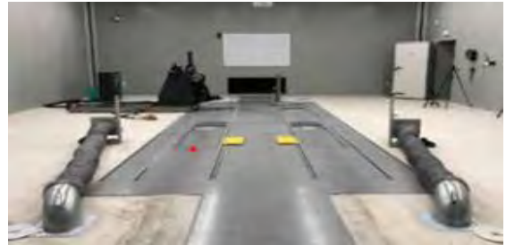
Fig. 1 Half-car module on roller bench in semi-anechoic
