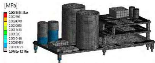
Fig. 2 A stress distribution diagram of the PCB assembly
