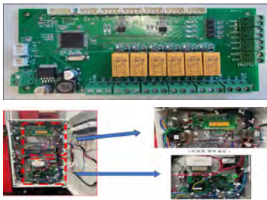
Fig. 1 Lift control board
