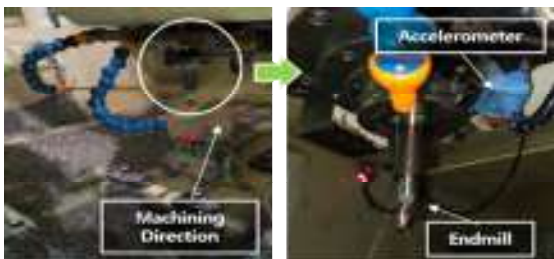
Fig. 1 Experimental setup and testing for monitoring
