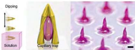
Fig. 1 Microneedle array using capillary force and it has a air trap [1]
